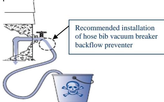
“Backflow” can happen if there is a water main break, water line repair, fire, or during a period of high water usage. These events may lower the pressure in the street enough to reverse the flow of water from your house. Also, if a pipe breaks inside a building, water can flow backwards from one room to another.
