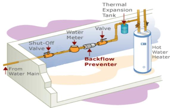
We may also require some residences to install a backflow prevention device at the meter, including any homes with a pool, a fish pond, lawn irrigation system or a private well on the property. These activities could contaminate the water mains if there was a backflow situation. If you are required to install a device, you will be responsible for the costs of materials, installation and testing.
